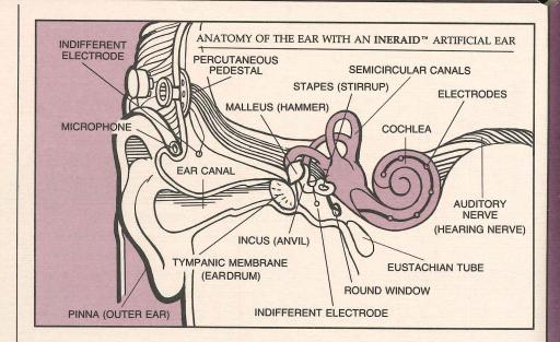
signals electromagnetically to a receiver implanted under the skin.
